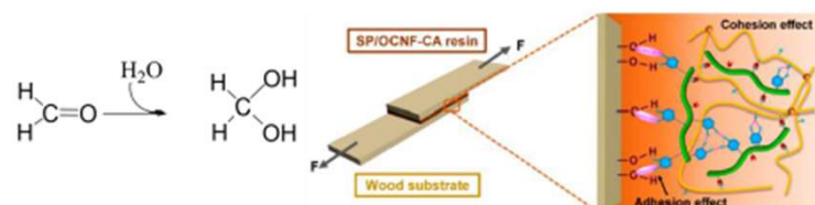
Figure 1. The application of hydrated formaldehyde (bio-resin) based materials for adhesion of wood. Adapted with permission from [5].
