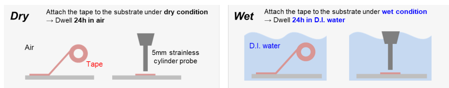
Figure 2-9. Test condition of evaluating adhesion properties
