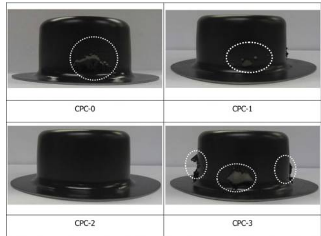
Figure 8 Formability of polyester coatings with long alkyl chains
