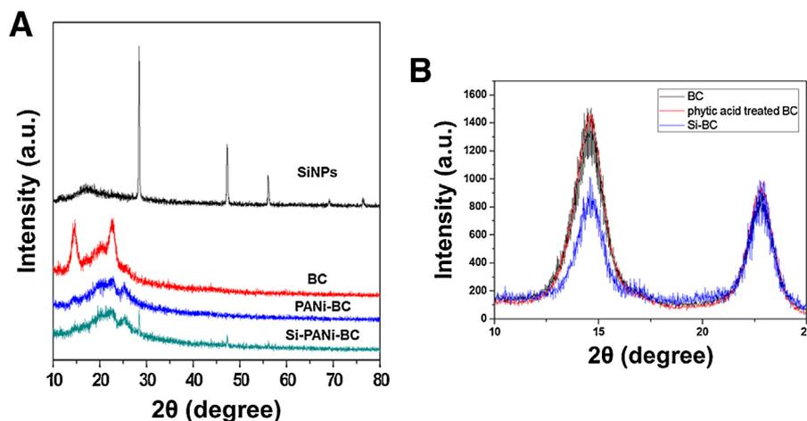
Fig. 5. XRD patterns of composites. (A) SiNPs, BC, PANi-BC, and PANi-Si-BC. (B) Change of crystallinity after the incorporation of SiNPs in BC.
