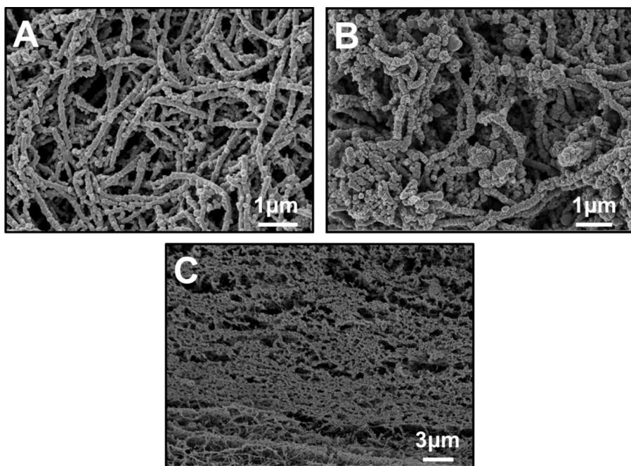
**Fig. 3.** SEM images of composites. (A) Surface image of PANi-BC, (B) surface image of Si-PANi BC, and (C) cross sectional images of freeze-dried PANi-Si-BC.
