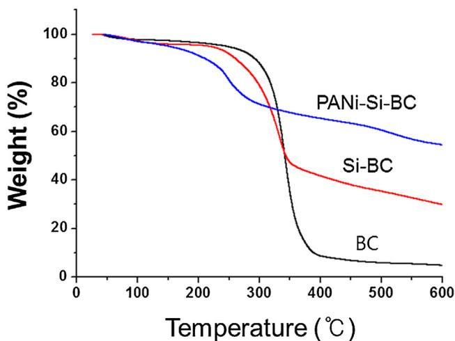
Fig. 6. Thermal stability of the composites. Thermogravimetric curves of BC, Si-BC and PANi-Si-BC were obtained using 10 mg of a vacuum dried sample in the range of temperature from 25 °C to 600 °C at a heating rate of 10 °C min<sup>-1</sup> under flowing nitrogen.
