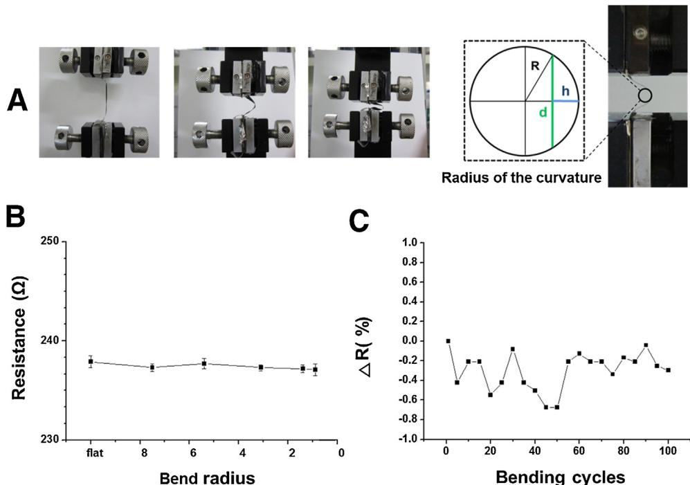
**Fig. 8.** Electrical stability of the composites to bending stress. (A) Optical images of bending process using UTM and parameters for the calculation of the bending radius, (B) resistance variation of PANi-Si-BC composite for changes in bending radius, and (C) the percentage of resistance change of the composite according to bending cycle up to 100 cycles.
