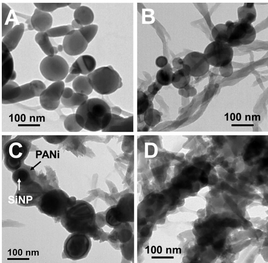
**Fig. 4.** TEM images of composites. (A) Si-BC and (B) Si-PANi without phytic acid. (C) Si-PANi and (D) PANi-Si-BC with phytic acid.
