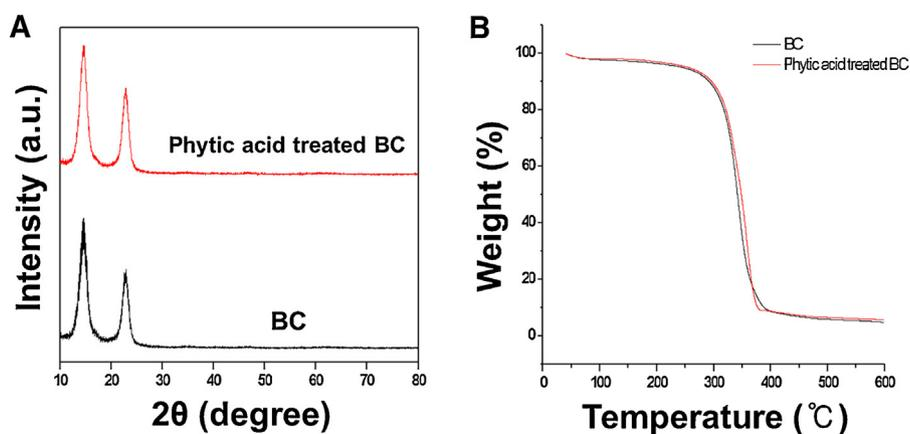
Fig. 7. Effect of phytic acid on the composites. (A) Morphological change and (B) the thermal stability of composites.
