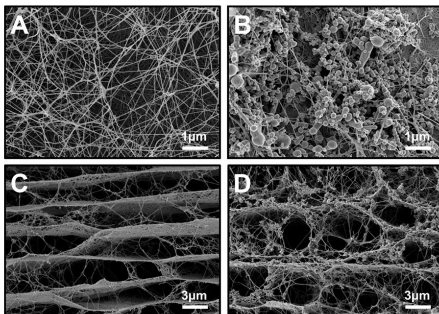
**Fig. 2.** FE-SEM images of BC and Si-BC composite. (A) Surface and (C) cross section of freeze-dried BC. (B) Surface and (D) cross section of freeze-dried Si-BC composite.
