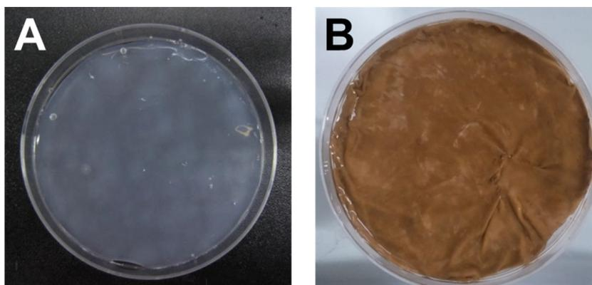
Fig. 1. Optical images of (A) pure BC and (B) Si-BC composite.
