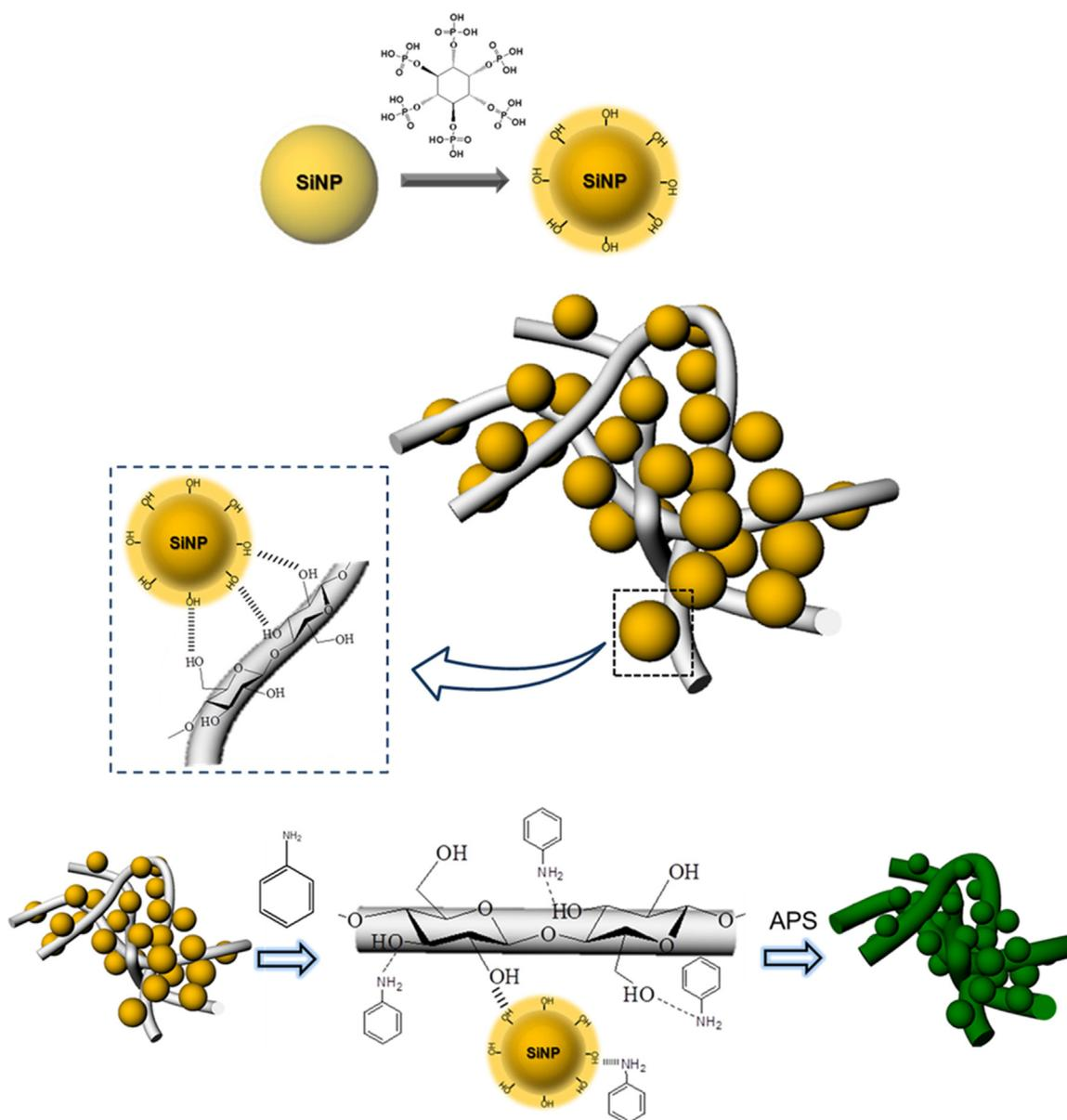
**Scheme 1.** Schematic representation of the process for preparing PANi-Si-BC composite. Hydroxyl groups were introduced on the surface of SiNPs as a result of modification with phytic acid. Hydroxyl groups of SiNPs can form hydrogen bonds with BC nanofibers. After adding aniline monomer and APS, PANi was polymerized on both BC nanofibers and SiNPs. The BC structure can serve as the template for both the adsorption of SiNPs and the polymerization of PANi.
