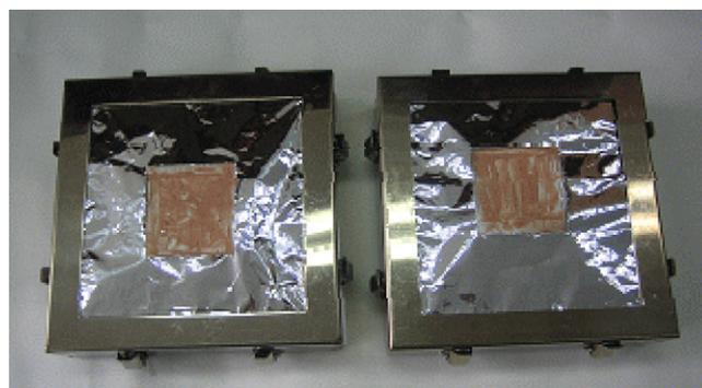
**Fig. 1.** Examples of glass plates coated with paint.
