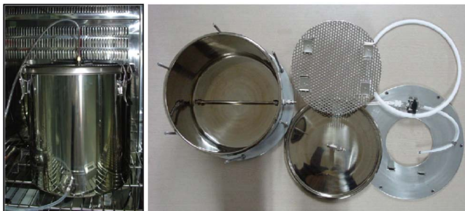
Fig. 2. The 20 L small chamber.
