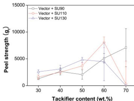
**Figure 11** Peel strength of Vector/tackifier as a function of tackifier content. [Color figure can be viewed in the online issue, which is available at [www.interscience.wiley.com](http://www.interscience.wiley.com).]
