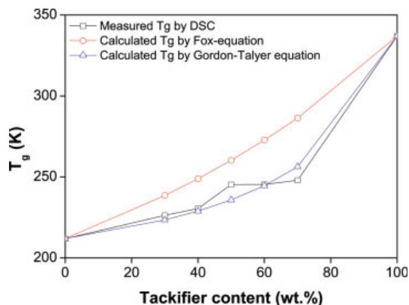
**Figure 7** Comparison of  $T_g$  between  $T_g$  by DSC and  $T_g$  calculated by Fox-equation and Gordon-Talyer equation ( $\kappa = 0.2$ ). [Color figure can be viewed in the online issue, which is available at [www.interscience.wiley.com](http://www.interscience.wiley.com).]
