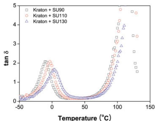
**Figure 6** The  $\tan \delta$ -temperature curves of PSA as a function of  $T_g$  of tackifier. [Color figure can be viewed in the online issue, which is available at [www.interscience.wiley.com](http://www.interscience.wiley.com).]
