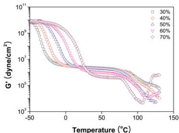
**Figure 2** Storage modulus–temperature curves of PSA as a function of tackifier content (Kraton : SU110). [Color figure can be viewed in the online issue, which is available at [www.interscience.wiley.com](http://www.interscience.wiley.com).]
