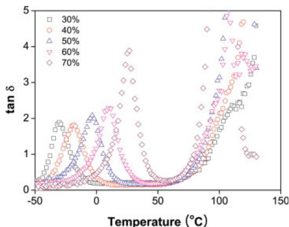
**Figure 4** The  $\tan \delta$ -temperature curves of PSA as a function of tackifier content (Kraton : SU110). [Color figure can be viewed in the online issue, which is available at [www.interscience.wiley.com](http://www.interscience.wiley.com).]
