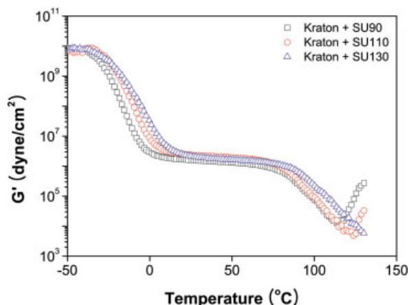
**Figure 5** Storage modulus-temperature curves of PSA as a function of  $T_g$  of tackifier. [Color figure can be viewed in the online issue, which is available at [www.interscience.wiley.com](http://www.interscience.wiley.com).]
