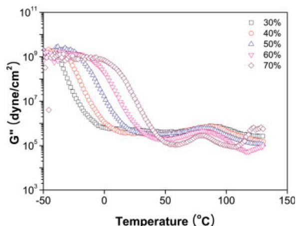
**Figure 3** Loss modulus–temperature curves of PSA as a function of tackifier content (Kraton : SU110). [Color figure can be viewed in the online issue, which is available at [www.interscience.wiley.com](http://www.interscience.wiley.com).]
