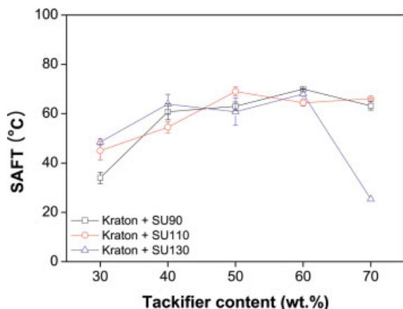
**Figure 12** SAFT of Kraton/tackifier blends as a function of tackifier content. [Color figure can be viewed in the online issue, which is available at [www.interscience.wiley.com](http://www.interscience.wiley.com).]
