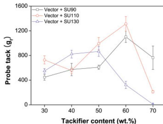
**Figure 9** Probe tack of Vector blends as a function of tackifier content. [Color figure can be viewed in the online issue, which is available at [www.interscience.wiley.com](http://www.interscience.wiley.com).]
