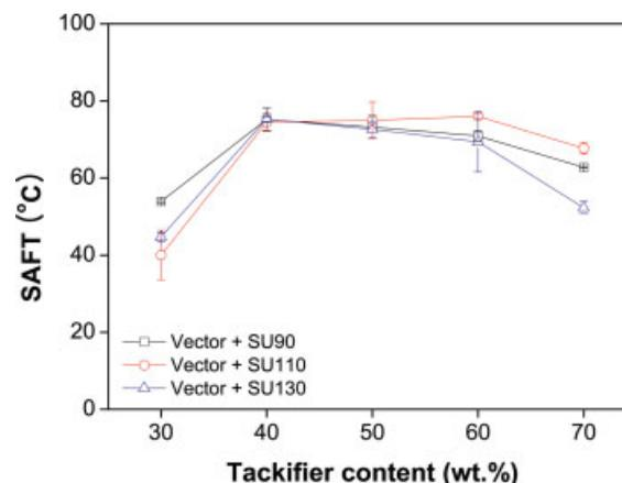
**Figure 13** SAFT of Vector/tackifier blends as a function of tackifier content. [Color figure can be viewed in the online issue, which is available at [www.interscience.wiley.com](http://www.interscience.wiley.com).]
