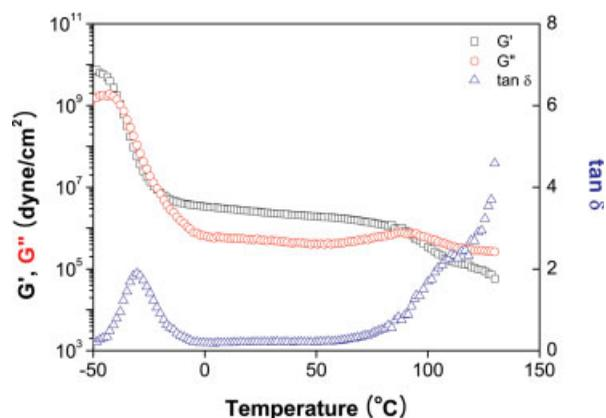
**Figure 1** Viscoelastic property–temperature curves of PSA (Kraton : SU110 = 7 : 3). [Color figure can be viewed in the online issue, which is available at [www.interscience.wiley.com](http://www.interscience.wiley.com).]
