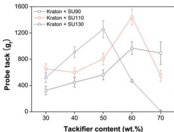
**Figure 8** Probe tack of Kraton blends as a function of tackifier content. [Color figure can be viewed in the online issue, which is available at [www.interscience.wiley.com](http://www.interscience.wiley.com).]
