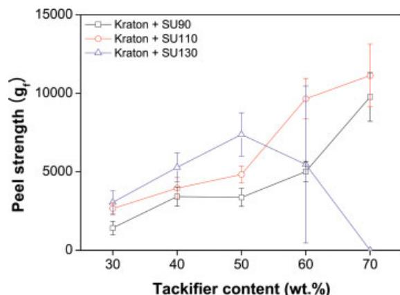
**Figure 10** Peel strength of Kraton/tackifier as a function of tackifier content. [Color figure can be viewed in the online issue, which is available at [www.interscience.wiley.com](http://www.interscience.wiley.com).]
