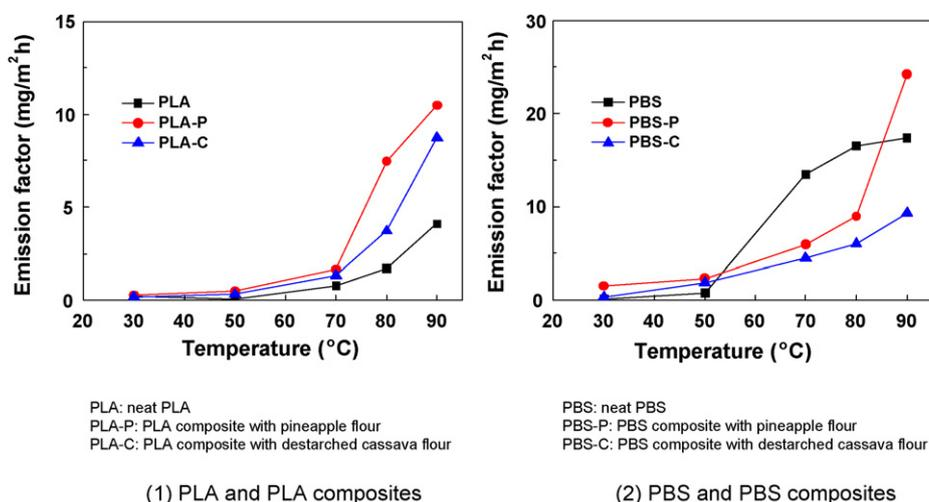
Fig. 2. TVOC emission factors of the PLA, PLA composites, PBS and PBS composites.
