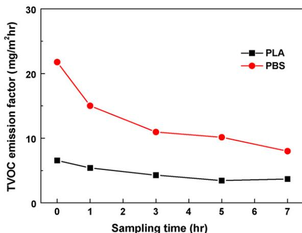
Fig. 3. TVOC emission factors as a function of the baking time.
