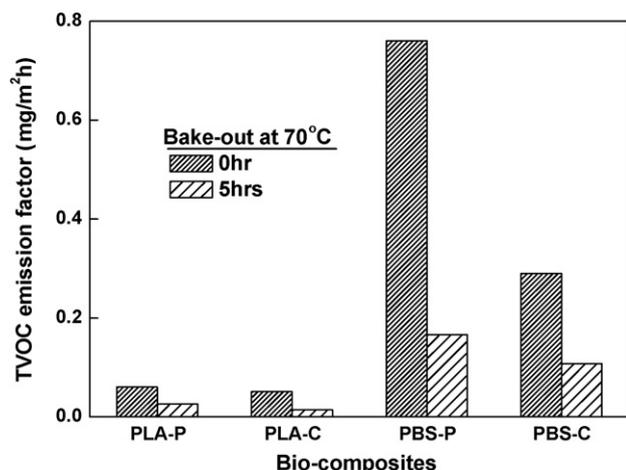
**Fig. 9.** TVOC emission factor of PLA and PBS composites using a 20L small chamber.
