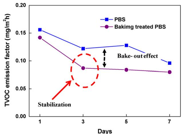
Fig. 8. TVOC emission behavior of PBS using a 20L small chamber.
