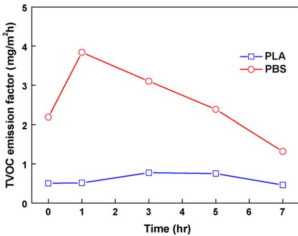
Fig. 5. TVOC emission factor using FLEC (at 70 °C).
