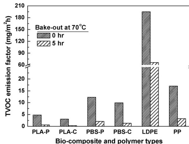
Fig. 4. Bake-out application for the PLA composites, PBS composites, LDPE and PP.
