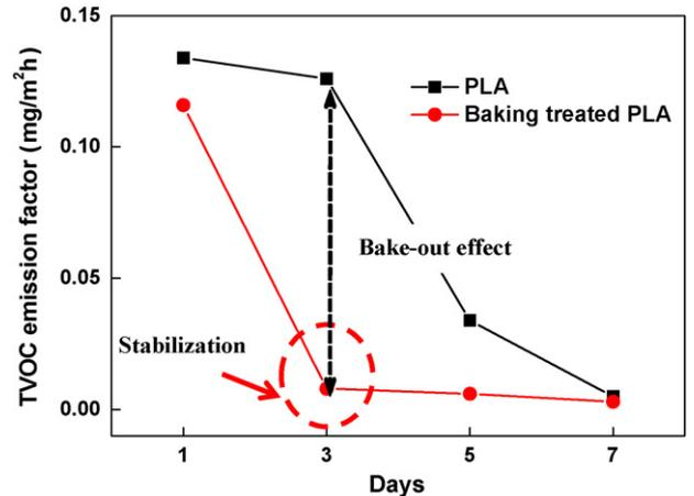
Fig. 7. TVOC emission behavior of PLA using a 20L small chamber.
