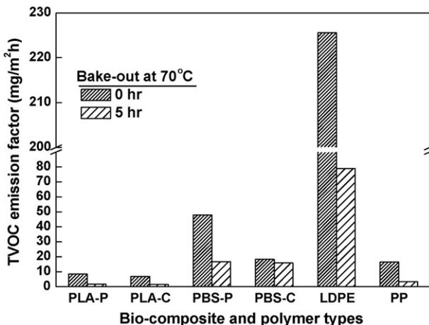
Fig. 6. Bake-out application for the PLA composites, PBS composites, LDPE and PP using FLEC.
