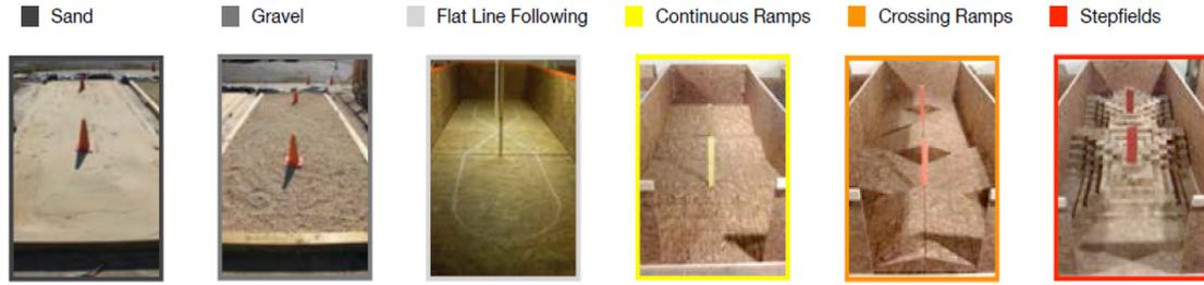
Fig. 4. Classification the ground state of failure factor for robot operation (NIST, 2014).
