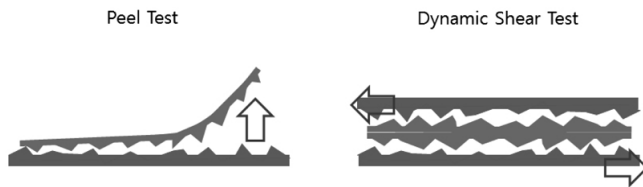
Figure 7. Mechanism of peel and dynamic shear test.
