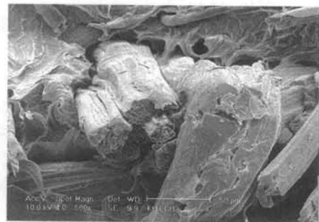
Fig. 14. SEM micrographs of PP/5% NaOH treated kenaf fiber (70/30) interface on composite :50 \mu\text{m} (at 500 \times ).
