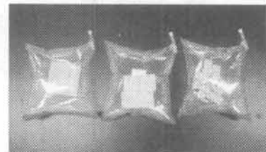
Figure 2. Three kinds of specimens with N 2 in 3L polyester bag.
