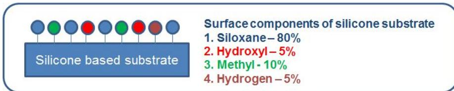
Figure 8. Surface characteristics of silicon substrate and additional approach of silicone functionality to acrylic back bone
