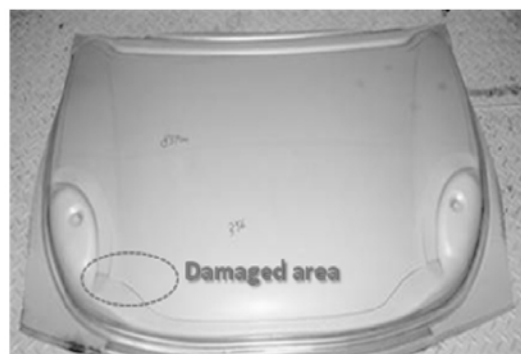
Figure 8. Surface deformation of coatings after forming process.
