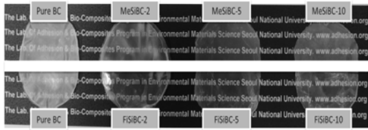
Figure 10. Photograph of optically transparent BC/GPTMS composite film fabricated according to GPTMS concentrations[28].
